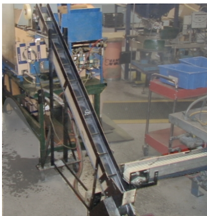
Homemade, inexpensive inclined conveyor to bring products up to working height.
