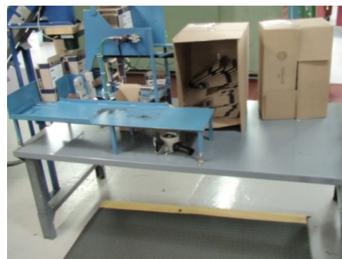
Packing station (opposite view of photo at left). Features include automatic counting system, cylinders to push product boxes into position, and a two-tiered packing station to reduce arm motions when loading product boxes into shipping boxes.
