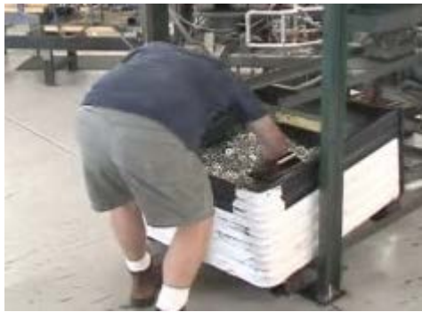
Before: Bending low into a bin to scoop out parts and then reaching high to dump them into a hopper.
