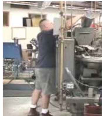
Before: Bending low into a bin to scoop out parts and then reaching high to dump them into a hopper.
